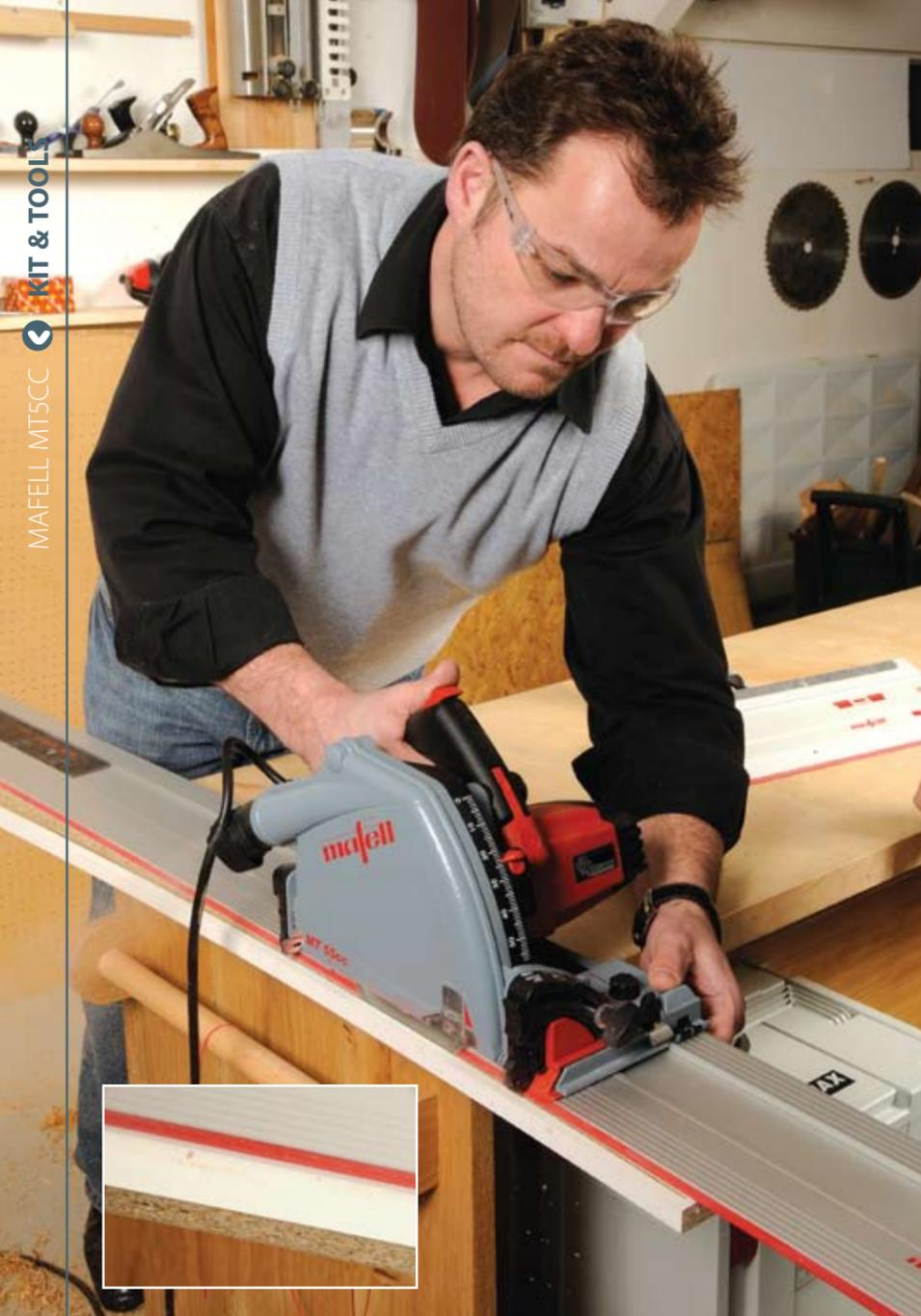
We were absolutely blown away by the ingenuity of the cleverly-angled scoring cut that's built into the saw. It left melamine absolutely splinter free!
