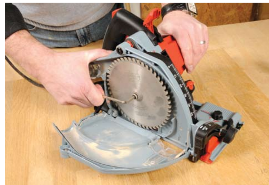
It took literally seconds to change between the two included blades, with no danger to the user and a snap in, snap out approach that won't hinder the worker under pressure
