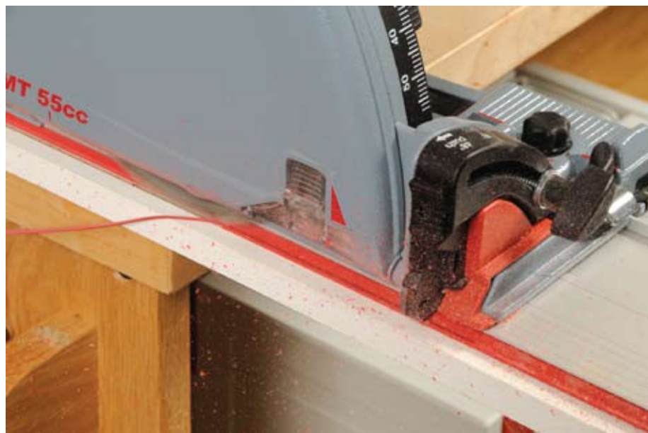
Here we are taking the rubbery protective coating off the edge of the guide rail for the first cut, soon to make short work of the tricky melamine
