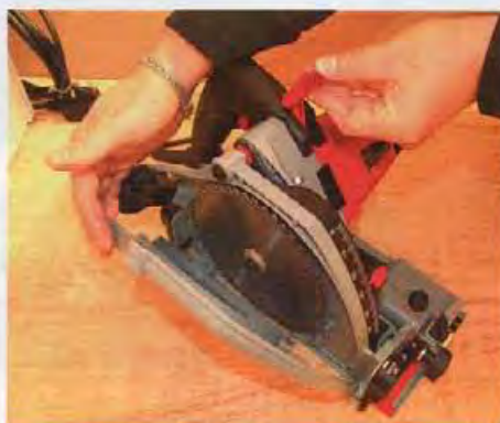
▲ Pic.8 Lifting this lever drops the flap automatically for blade changing. It locks the spindle and trigger at the same time
