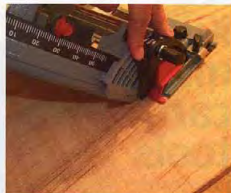
▲ Pic.3 Lifting the lever drops the flap automatically for blade changing. It locks the spindle and trigger at the same time
