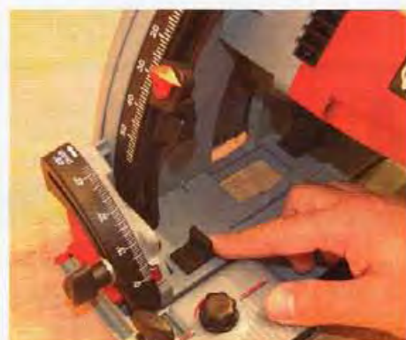
▲ Pic.6 This button lets the saw tip inwards by 1° for slight undercutting
