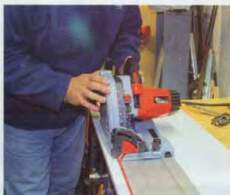
▲ Pic.5 The scoring facility on melamine is excellent, the initial score cut fractionally offset
