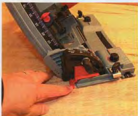
▲ Pic.7 As the blade angle alters, this cursor slides out to indicate the kerf position
