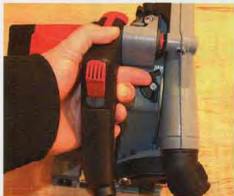
▲ Pic.1 Sliding this button across limits the plunge for pre-scoring, giving very clean cuts in veneered and melamine stock
