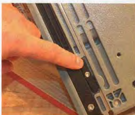
▲ Pic.11 Here you see the insert that tightens the fit to the rail
