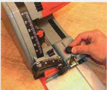
▲ Pic.10 The fit to the rail is snugged up with small offset cam knobs
