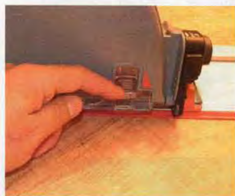
▲ Pic.9 Sliding this cover down increases the suction around the blade to keep the cut line quite clear
